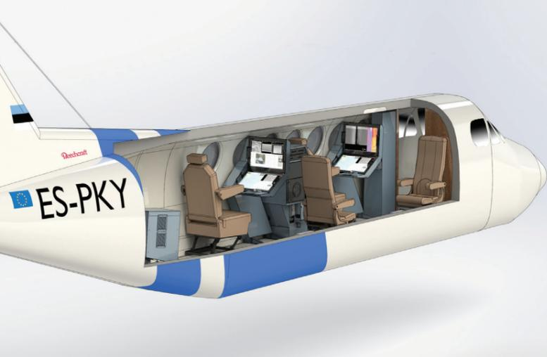
The MSS 7000 equipped aircraft provides a superior working environment. Ergonomic seats are installed for two system operators and two observers. Two identical consoles allow the two operators full flexibility in sharing the work load between themselves.
