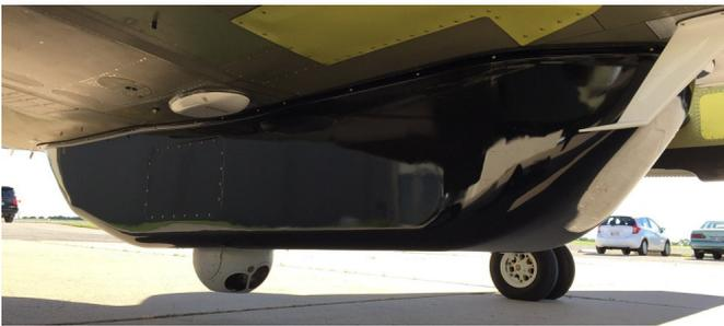
Photo of the radome as fitted on the aircraft, just before the first test flight.
