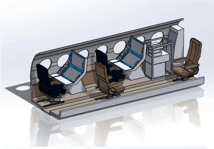
The MSS 7000 equipped aircraft provides a superior working environment. Ergonomic seats are installed for two system operators and two observers. The operator consoles have been designed to give the operator immediate access to all functions of the system. Two identical consoles allow the two operators full flexibility in sharing the work load between themselves. A full communications suite ensures real time coordination with cooperating units and mission command at all times.
